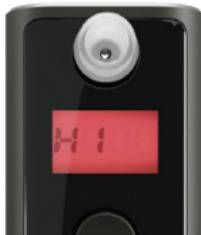
The measurement result exceeds the measurement range of the device.
