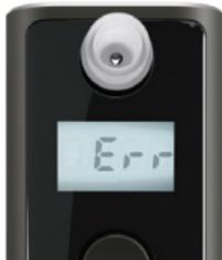
Provided air sample is too small. Perform the measurement again providing a strong and steady exhalation.
