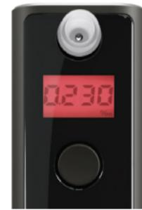
The device is ready to take an air sample. Take a deep breath and blow into the mouthpiece for approx. 6 sec. The device will emit an intermittent beep while the sample is being taken.
