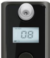
Low voltage. Replace the batteries.
