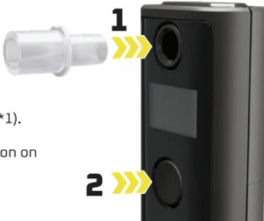
Insert the mouthpiece into the measuring hole (\*1).
