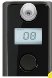
After starting, you will hear a single beep. The display will show four eights (\*1), and then the breathalyzer will display the number of measurements already taken (\*2) and start preparing for the test by counting down from 10 to 0 (\*3).
